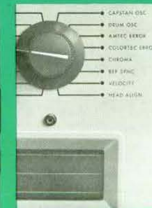
Important VTR circuits fully monitored with built-in A-Scope.
