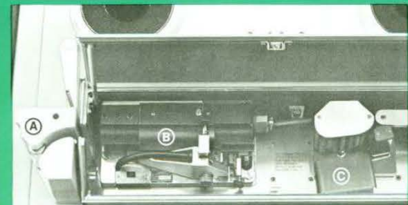
Easy-to-load tape path contains: (A) new non-scratch video erase head, (B) Mark Ten video head with rotary transformer coupling... interchangeable with other Ampex VTR's via plug-in modules, (C) new flip-down audio head shield for easy cleaning.
