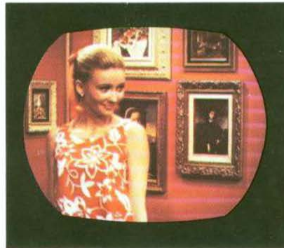
Velocity Compensator "out-of-circuit" during replay of tape; velocity error.
