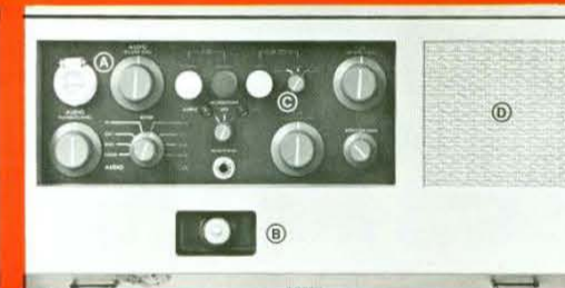
New, audio/cue system has: (A) "spot erase" feature, (B) built-in dynamic mike, (C) switchable cue tone oscillator, (D) built-in speaker plus high-fidelity output for external speaker.
