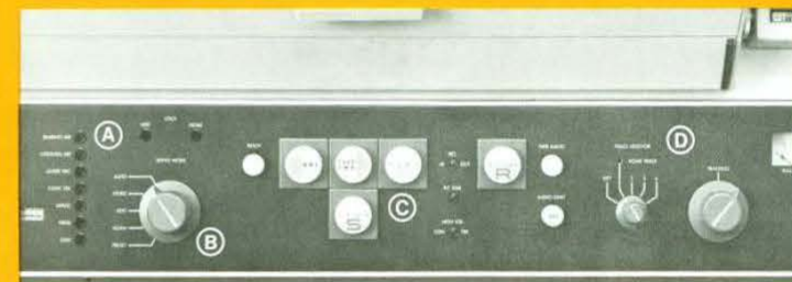
Logically arranged panel features: (A) full protection at-a-glance with meaningful CAUTION, OK and WARNING lights... plus other fail-safe features, (B) complete front panel servo mode control, (C) centralized, interlocked controls for convenient and error-free operation, (D) front panel control and meter indication of all four tracking modes.
